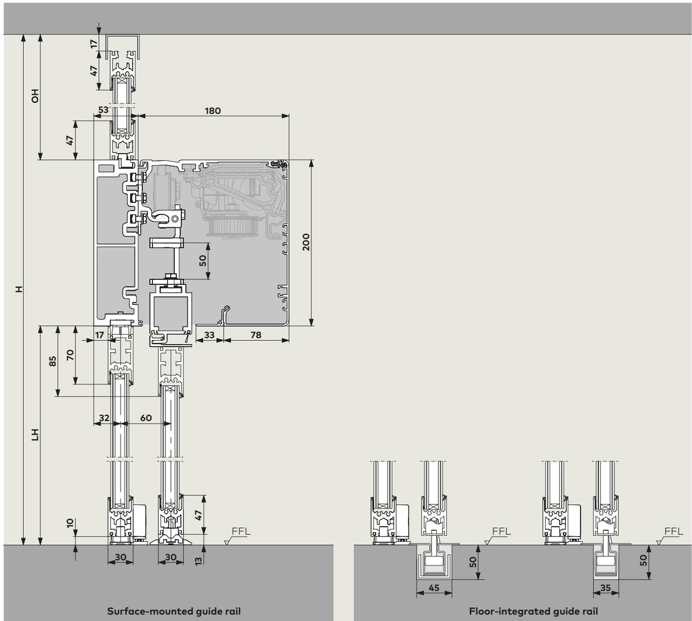
Double-panel version with surface-mounted guide rail
