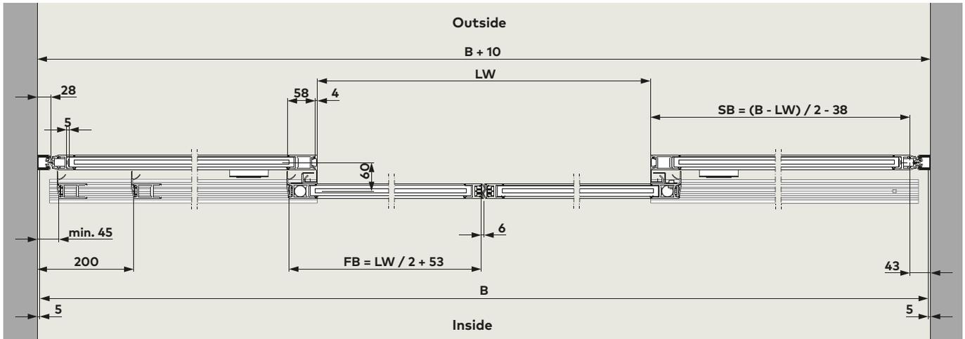
Double-panel version with floor-integrated guide rail
