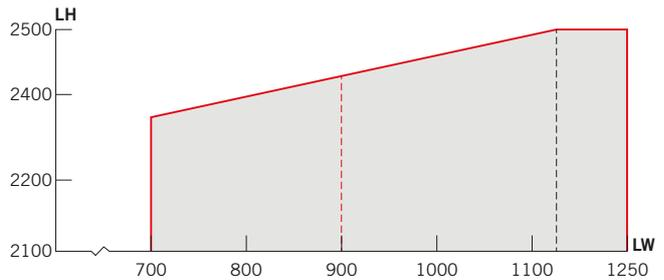
Escape route systems must have a minimum clear passage width of 900 mm!
