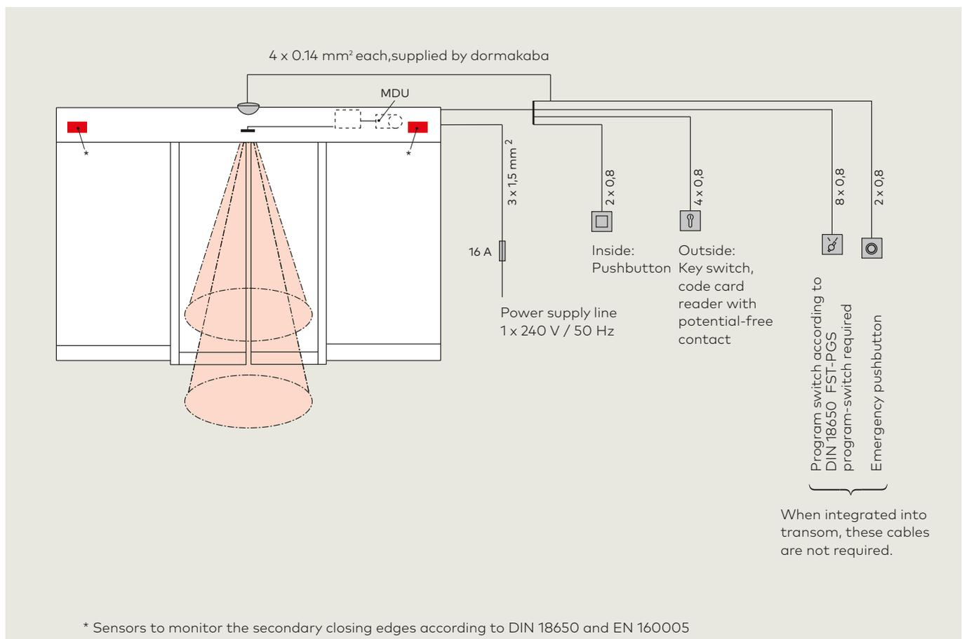
The external emergency pushbutton has to be installed in the close range of the door. Max. cable length: 50 m.
